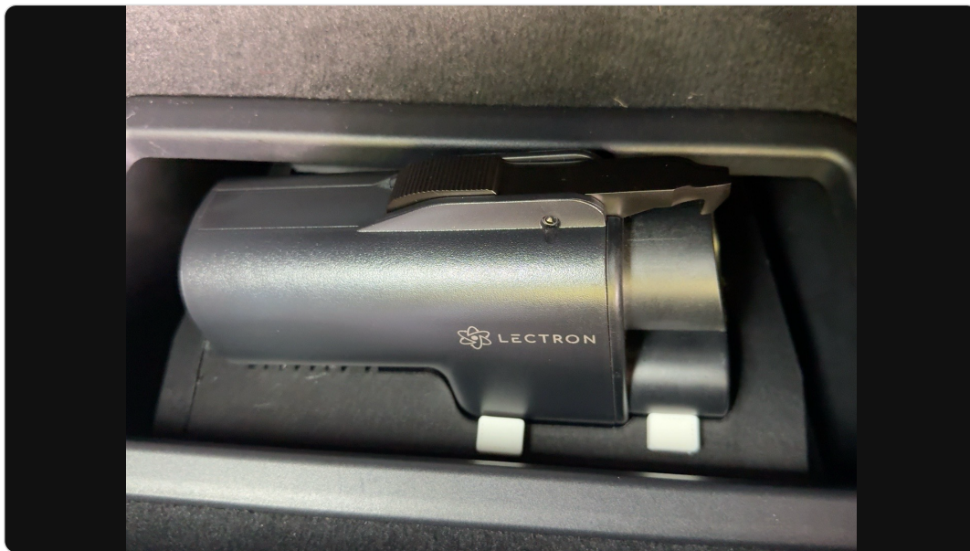
Final installed orientation with the Lectron adapter seated in the carrier.
