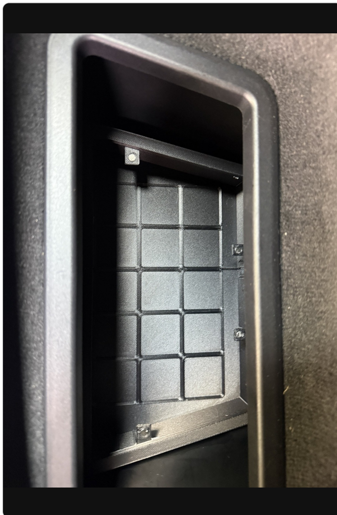
Correct final position: lower tray fully seated on the cubby floor.
